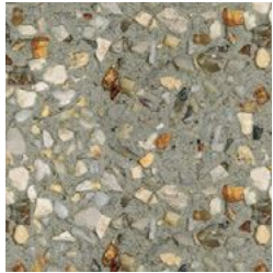
shared path_ washed aggregate concrete
