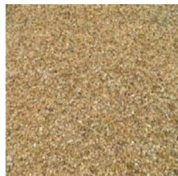
surface treatment_ stabilised gravel
