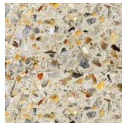
shared path_ washed aggregate concrete
