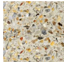
shared path_ washed aggregate concrete
