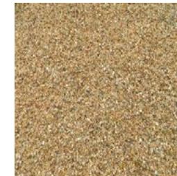
surface treatment_ stabilised gravel
