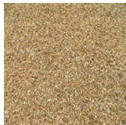
surface treatment_ stabilised gravel
